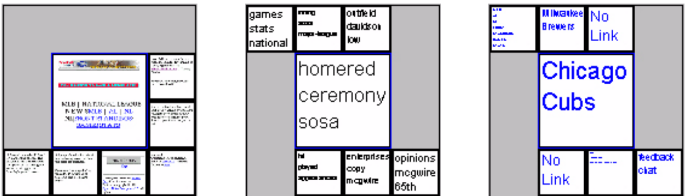
Figure 4. The Web browser of Small Terminals (WEST). All three views are shown in their actual resolution of 160*160 pixels. The views are, from left to right, the thumbnail view, the keyword view and the link view.
