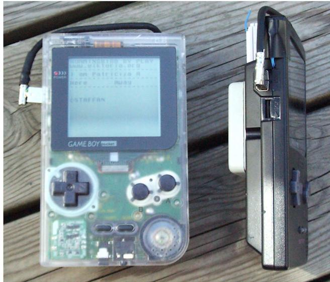
**Figure 2:** Picture showing the Generalised Hummingbirds, i.e., GameBoys fitted with radio transceivers.
